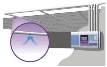
A centralized VESDA detector draws air through a simple pipe network installed in the ceiling space.
